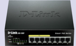
Network Switch Transmitting camera visuals to a laptop Providing an interface for camera control
